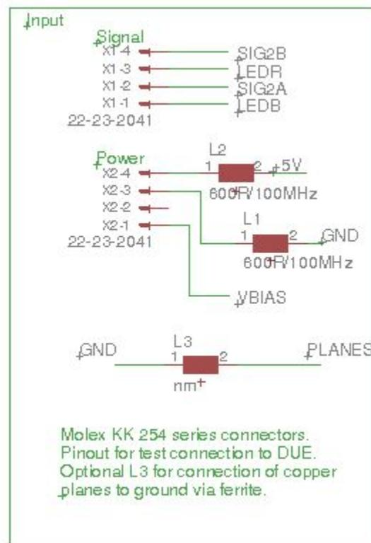
Figure 2: Input and Output connections from the Analogue Board
