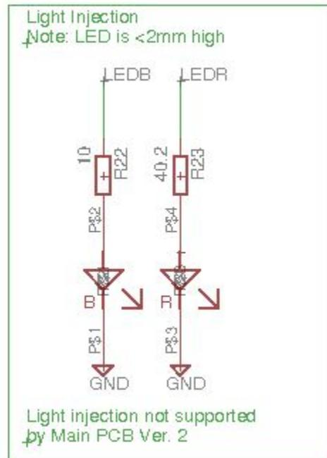
Figure 7: LEDs for Light Injection
