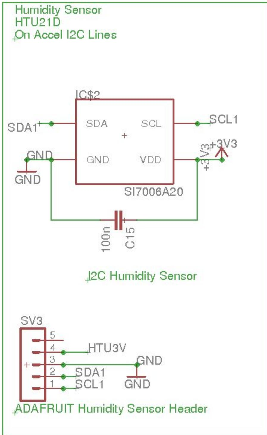
A humidity sensor is provided to help track the ageing of the plastic scintillator. There are numerous papers which indicate that the presence of humidity has a negative effect on the lifetime performance of certain types of scintillator medium, therefore a sensor has been included to assist in checking the quality of the environment within
