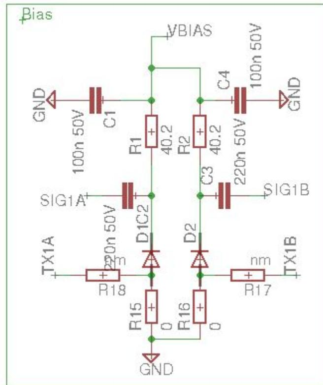
Figure 3: Bias configuration for SiPMs
