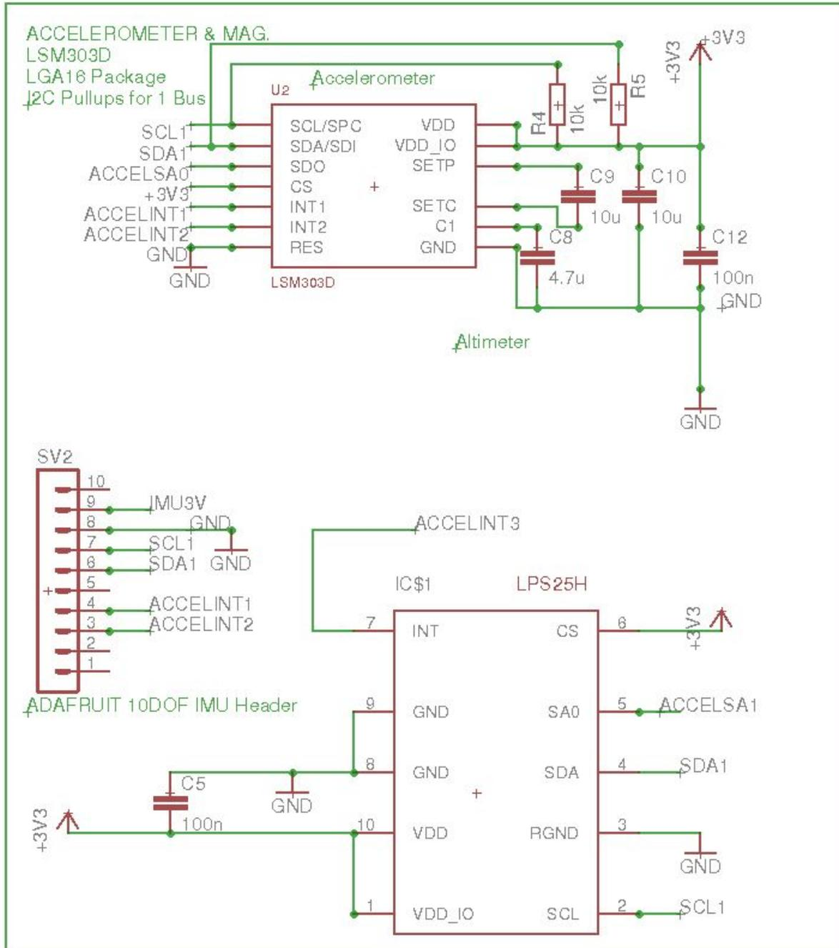
The Inertial Measurement Unit (IMU) is comprised of two discrete IC's which replicate the functionality of the Adafruit 10DOF IMU header. A 10 pin 2.54mm pitch
