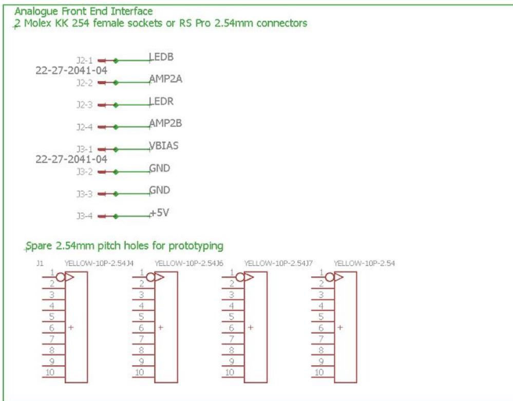
Two four pin headers are provided for connection to the Analogue Board. In version 2 alpha main boards, only 5 signals are connected to these headers (AMP2A, AMP2B, VBIAS, GND and +5V). Version 2.1 adds two additional signals LEDB and LEDR, to permit light injection testing if a suitable LED is installed on the analogue board. The headers are standard 2.54mm type and are fixed on the upper face of the PCB to allow the analogue board and scintillator module to be stacked on top.
