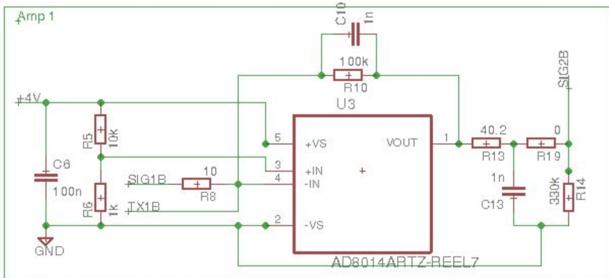
Figure 5: Amplification and shaping stage
